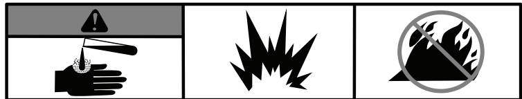
Battery acid is corrosive, explosive and flammable
