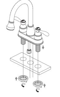
**3** Attach lower end of spray hose to central supply tube in facuet.
