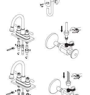
**5** Wrap supply inlets with pipe tape and connect to water supply.
