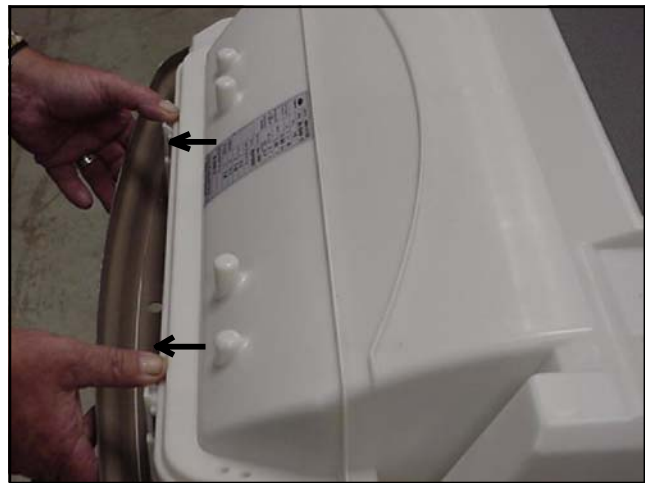
Figure 3-29 Upper Scroll Assembly Keeper Tab Release
