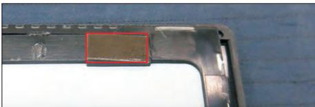
Use a Philips-head screwdriver to remove 2pcs screws for unlocking the front bezel with the panel module, and then use a proper tool to disconnect the panel lamp cable, LVDS cable and function key board from the connector of the main board.
