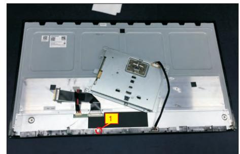
Put the front bezel with function key board into a fixture, tear off the mylar, then use a Philips-head screwdriver to remove 3pcs screws for unlocking the function key board with front bezel.
