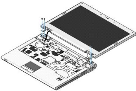
6. In sequential order, remove the four numbered M2.5 x 5-mm screws from the base of the display assembly.
