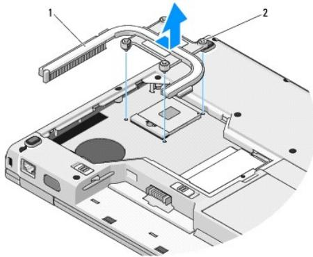
1 processor thermal-cooling assembly 2 captive screws (4)
