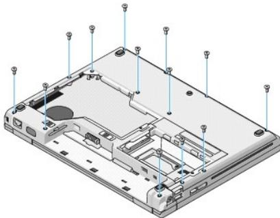
9. Turn the computer over and remove the nine M2.5 x 5-mm screws and two M2 x 3-mm screws that secure the top of the palm rest.
