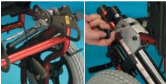
Front and rear transport tie down brackets are mounted where caregivers can reach.**
