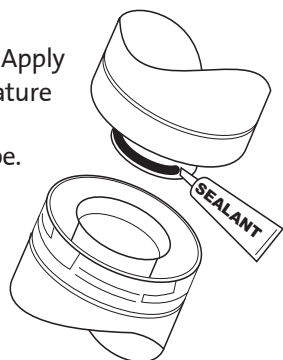
Figure 9. Seal each inner joint before joining pipe.
