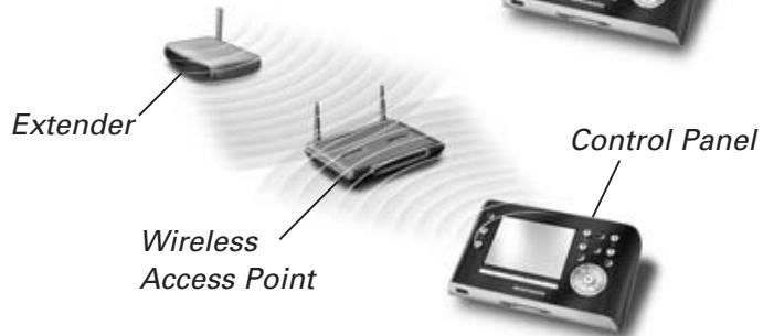
**Note** When you set up a Wireless **Wizz.Ex** Network connection, make sure the Control Panel always shows minimal one bar of WiFi connectivity. If this is not the case, you may need additional Wireless Access points in your network.
