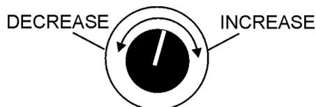
Figure 9. Voltage Regulator Control Knob
