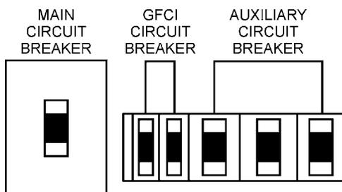
**Figure 52. Main, GFCI and Load Circuit Breakers Off**
