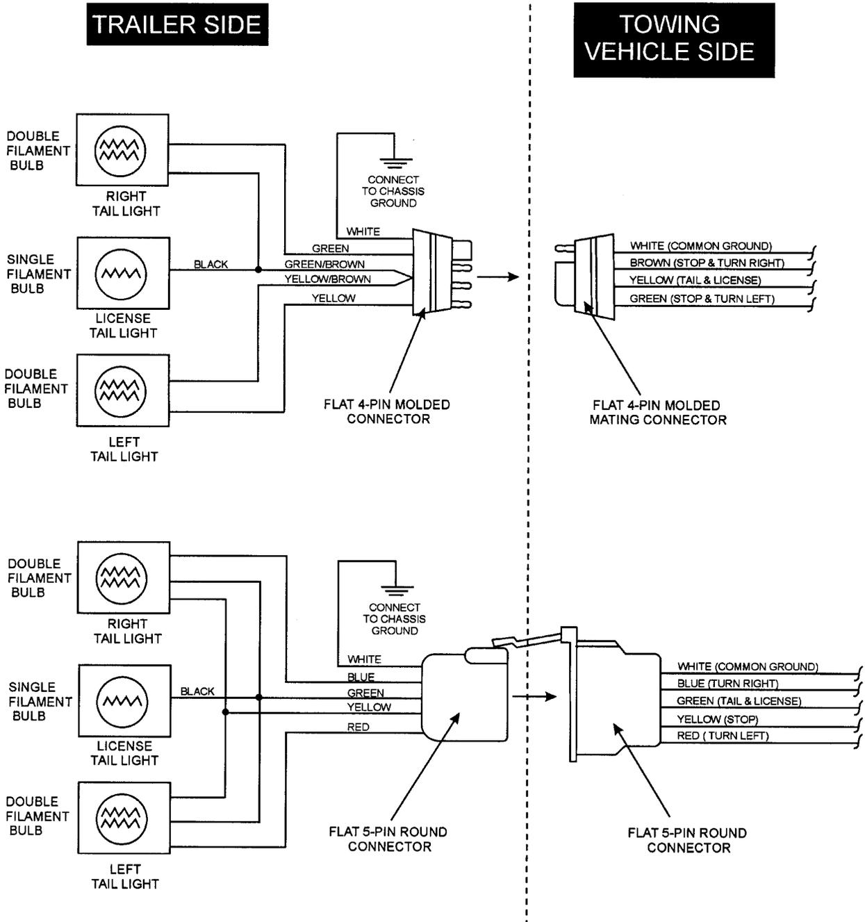
Figure 61. Trailer/Towing Vehicle Wiring Diagram
