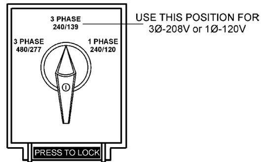
**Figure 22. Voltage Selector Switch
