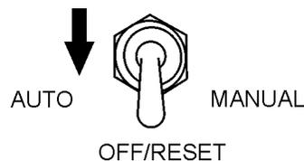
**Figure 54. MPEC Control Switch (Off/Reset)**
