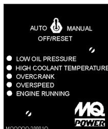
If the engine does not engage (start) by the third attempt, the engine will be shutdown by the engine controller's Over Crank Protection mode. If the engine engages at a speed (RPM's) that is not safe, the controller will shutdown the engine by initializing the Over Speed Protection mode.
