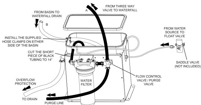
REMOVE COMPONENTS FROM BASIN AND ASSEMBLE AS SHOWN. THE FITTINGS REQUIRED ARE ALREADY ATTACHED TO THE FILTER AND BASIN. MEASURE AND CUT THE LINES TO THE LENGTH NECESSARY, PUSH ONTO THE BARBED 10 FITTINGS AND SECURE WITH THE SUPPLIED HOSE CLAMPS. LEAK TEST THE WATERFALL BEFORE FULLY ENCLOSING.
