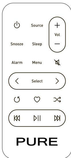
⏮ and ⏷ Skip to start of current track or go to previous/next track. Hold to fast rewind or fast forward.
