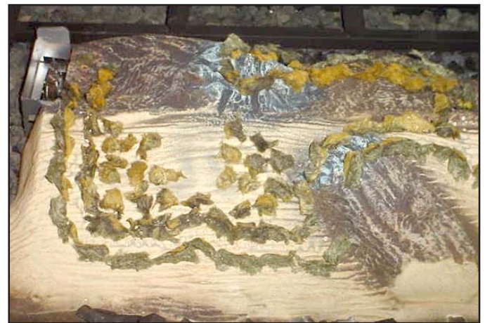
Figure 53. Placement of the Ember Material
