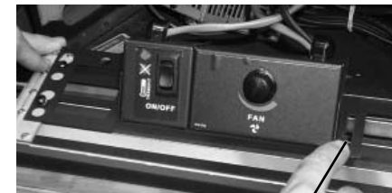
Hold control box assembly in place and mark the position of the right side slot
