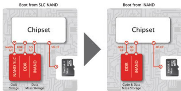
Because iNAND-based MCP devices of various configurations, capacities and package sizes share the same architecture and ballout, one platform design can be used for various handset models.
