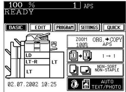
**4** Press either **(◀)** or **(▶)** key to adjust the copy density to the desired level.
