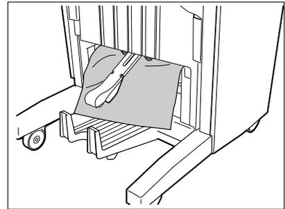
**7** Open the exit cover of the saddle stitch unit and remove any misfed paper.
