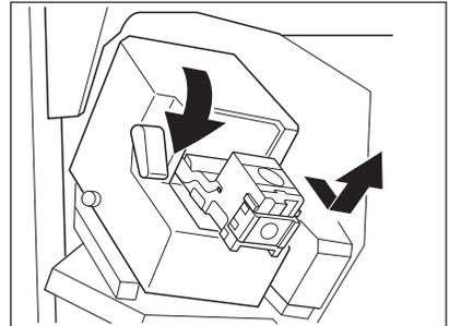
**3** Remove the empty staple case upward from the staple cartridge.
