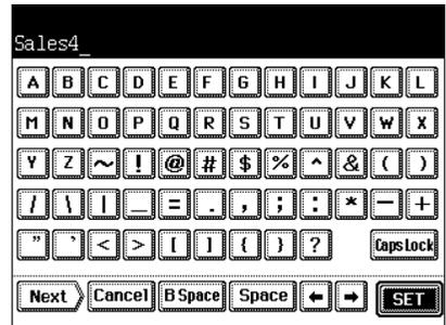
**5** Key in the desired account number (the same number) both for “NEW NUMBER” and for “RETYPE THE NEW NUMBER”, and press the lower **SET** key.
