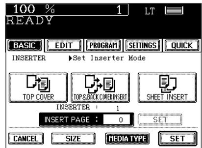
**8** Press the key of the paper size placed in the inserter, then press the **RETURN** key.
