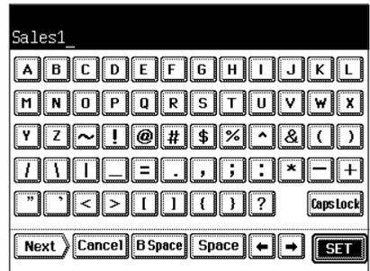
**6** Key in the desired master number (the same number) both for “NEW NUMBER” and for “RETYPE THE NEW NUMBER”, and press the **SET** key.
