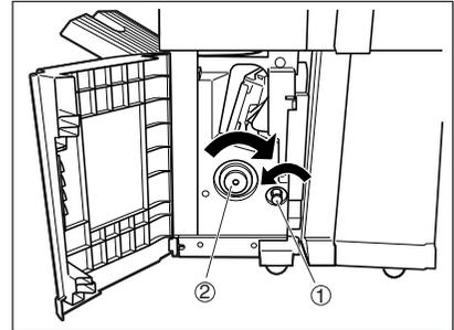
**6** Remove any paper misfed on the exit side of the saddle stitch unit.
