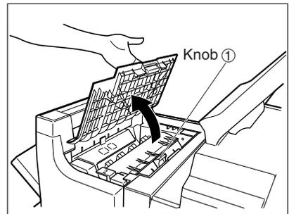
**7** **2** Lift knob **①** (See the upper right figure), then remove any misfed paper.
