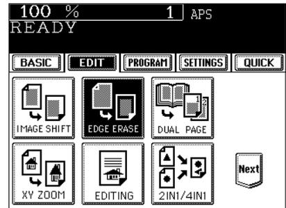
**4 Adjust the width of the white border, then press the **SET** key.**
