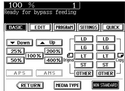
**3** Key in each dimension (length and width), or recall the data stored in the MEMORY. Then press the lower **SET** key.
