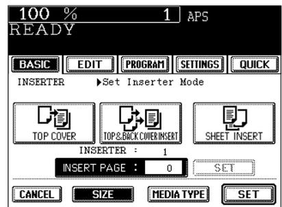
**6** Press the key of the paper size placed in the inserter.
