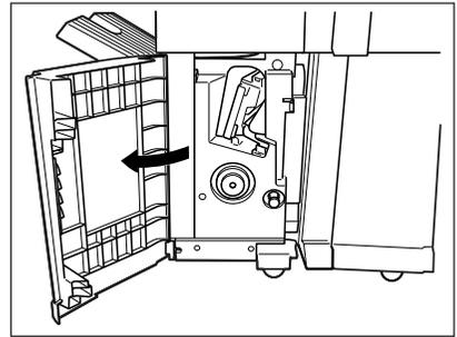
**5** Turn the right-hand knob ① counter clockwise. Then, push the left-hand knob ② and turn it clockwise.
