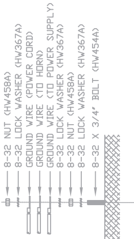
GROUND STUD DETAIL
