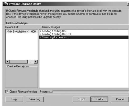
6. After reading the license agreement, click on the **I Agree** option and click **Next**. The *Firmware Upgrade Utility* main screen appears and displays the KVM switch in the *Device List* on the left side of the screen.
