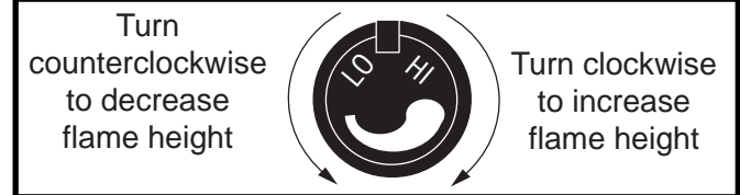
Fig. 20 Flame adjustment knob for Honeywell Valve.
