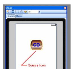
A source icon will appear on the Dragon 2.1 XTR39 computer screen. Double-click with the new source icon. A new page will appear showing the controls for the source component.
