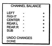
LEFT will be highlighted. The < and > arrow buttons will decrease and increase LEFT channel level respectively. When you've completed this adjustment, scroll to RIGHT and, once again, use the < and > arrow keys until the RIGHT level is satisfactory. Continue through CENTER, REAR L, REAR R, and SUB.
