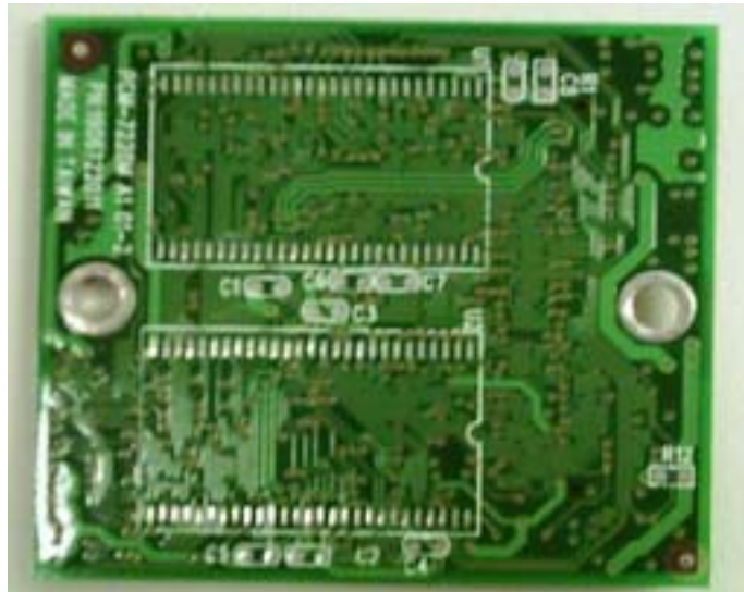
Figure 3.5 Solder side of Memory Module
