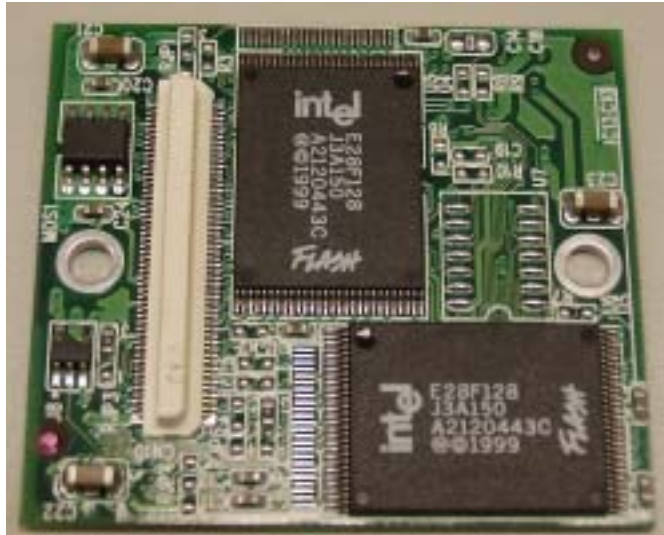
Figure 3.4: Component Side of Memory Module
