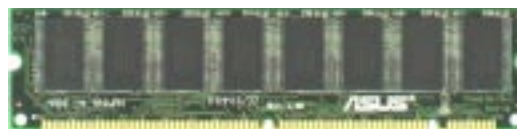
Non-ECC SDRAM DIMM (8 chips)
