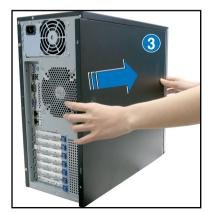
Drive in the two screws you removed earlier to secure the side cover.
