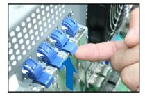
Remove the metal slot cover opposite the slot where you wish to install an expansion card.
