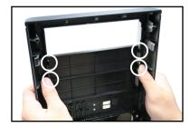
Unscrew and remove the metal cover of the bay where you want to install the 5.25-inch drive
