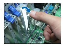
Align the card golden fingers with the slot, and then press firmly until the card is completely seated on the slot.
