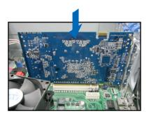
Restore the expansion card lock to its original position. A light click indicates that the card is locked in place.
