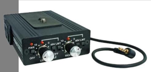
The BeachTek DXA-8 is a two channel, battery-powered microphone adapter with built in preamplifiers, limiters and dual phantom power. This adapter is designed to easily attach balanced or unbalanced type microphones to a consumer or prosumer camcorder. The DXA-8 gives you flexibility and control over the audio signal to ensure the best possible audio recording.
