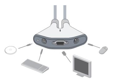
2. Connect the cables to the monitor, keyboard, and mouse ports on your two computers.
