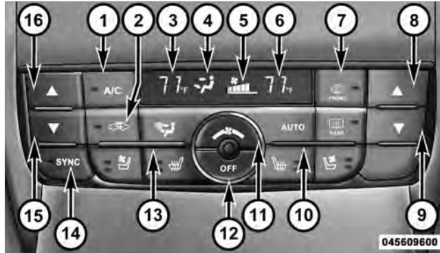
Automatic Temperature Control (ATC) Panel
