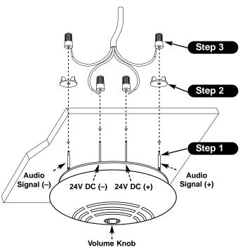
Set volume to maximum (1) before installation and adjust as needed
