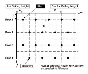
The layout of the speakers should be planned before installation begins. Layout starts in one corner of the room. The first speaker should be positioned from each wall a distance approximately equal to the ceiling height of the room.
