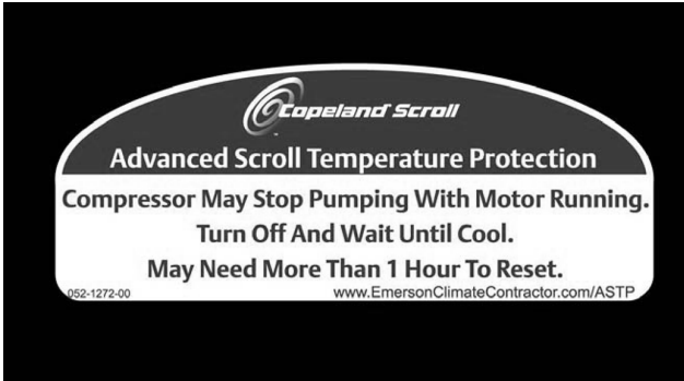
Fig. 14 — Advanced Scroll Temperature Protection Label
