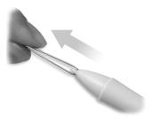
2. Firmly slide the new tip (square end first) into the barrel of the pen and press in until it stops.
