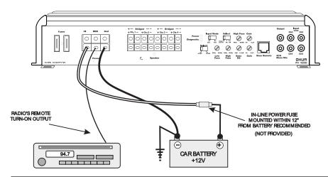
**IMPORTANT!** Before making any connections, disconnect the car's battery until the installation is completed to avoid possible damage to the electrical system.
