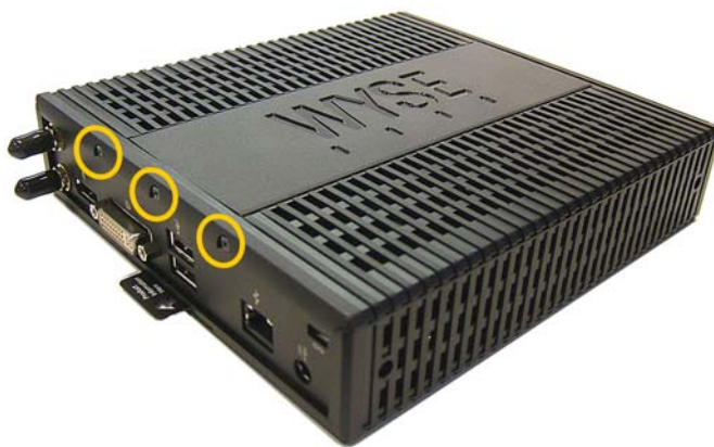
Figure 2 Removing the cover screws
