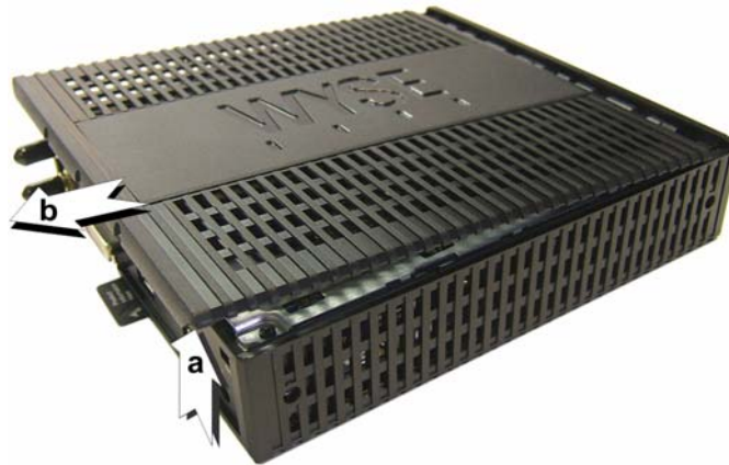
Figure 3 Removing the cover
