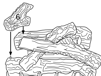
Figure 50 - Installing Log No. 6
