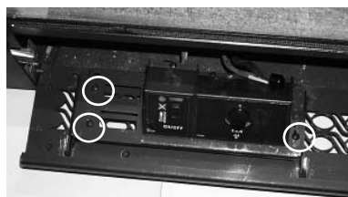
Secure left side with 2 screws and right side with one screw.
