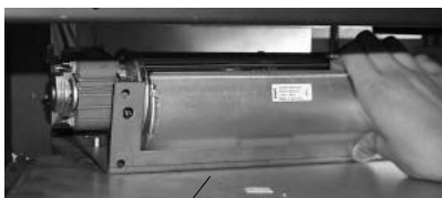
Position Fan B on mounting studs.
