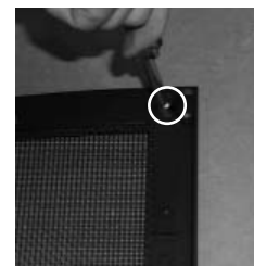
Loosen the screw holding the bracket.
