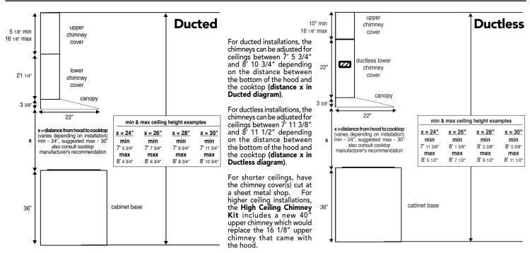
Note: If 24" or 30" High Backsplash is being installed, the distance between the bottom of the hood and the cooktop (distance x in diagram) is equal to the height of the Backsplash.
