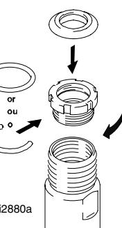
Loosely install packing nut onto cylinder.
