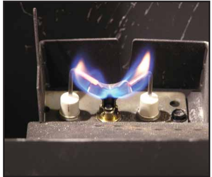
Figure 3.1 IPI Pilot Flame Patterns
