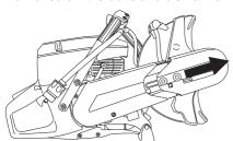
Remove the belt from the belt pulley.
