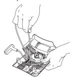
Remove any remnants of the old starter cord and check that the return spring works. Insert the new starter cord through the hole in the starter housing and in the cord pulley.
