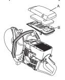
In order to obtain a good filtering effect, the filter must be replaced regularly or cleaned and oiled. A special HUSQVARNA oil has been produced for this purpose.
