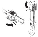
Press the power trigger and make sure it returns to its original position when you release it.
