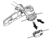
· Pull out the line chute assembly.
