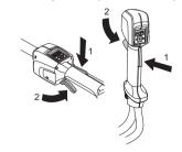
Make sure the power trigger is locked when the power trigger lock is in its original position.
